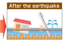
Fragmented grains of sand sink and cause water to emerge from the ground.
