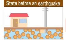
The grains of sand and the like stick to each other and there is water in between.
