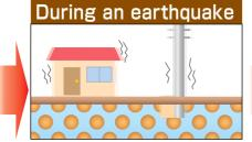
The grains of sand separate from each other and begin to float in the water.
