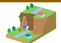
Cliff failures are a phenomenon where a steep slope of soil and sand collapses because of rainwater that has soaked into the ground during a heavy rain or the like.
